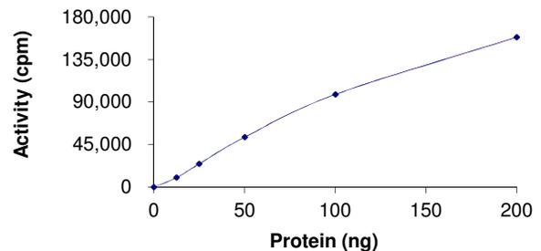
The specific activity of RET (V778I) was determined to be **56 nmol/min/mg** as per activity assay protocol.
