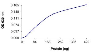
The specific activity of WIP1 was determined to be **151 nmol** /min/mg as per activity assay protocol.
