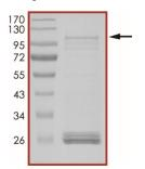
The purity of WIP1 was determined to be >70% by densitometry, approx. MW 110kDa.
