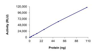
The specific activity of RIPK1 was determined to be 10 nmol/min/mg as per activity assay protocol.
