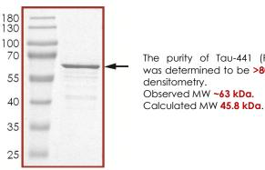
The purity of Tau-441 (P301S) was determined to be >80% by densitometry. Observed MW ~63 kDa.
