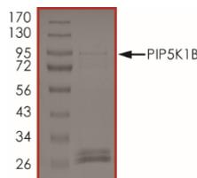
The purity of PIP5K1B was determined to be **>70%** by densitometry, approx. MW **96 kDa**.
