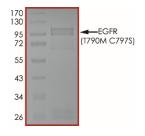
The purity of EGFR (T790M C797S) was determined to be >70% by densitometry, approx. MW 89~100kDa.
