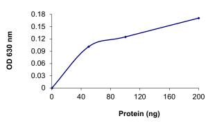
The specific activity of SHIP2 was determined to be 574 nmol phosphate released/min/mg as per activity assay protocol.
