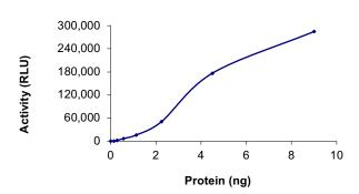
The specific activity of PAK3 was determined to be **56 nmol/min/mg** as per activity assay protocol.
