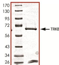
The purity of TRKB was determined to be **>80%** by densitometry, approx. MW **67kDa**.
