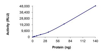
The specific activity of EGFR (d746-750 L718Q T790M) was determined to be **1.7 nmol/min/mg** as per activity assay protocol.
