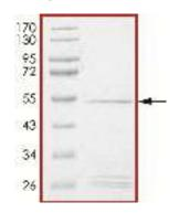
The purity of CyclinM was determined to be >90% by densitometry.
