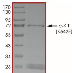
The purity of c-KIT (K642E) was determined to be **>75%** by densitometry, approx. MW **73 kDa**.
